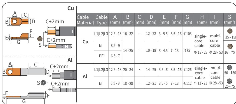
**Step 1:** Crimp the AC cable OT terminal, and prepare the AC output cable.
